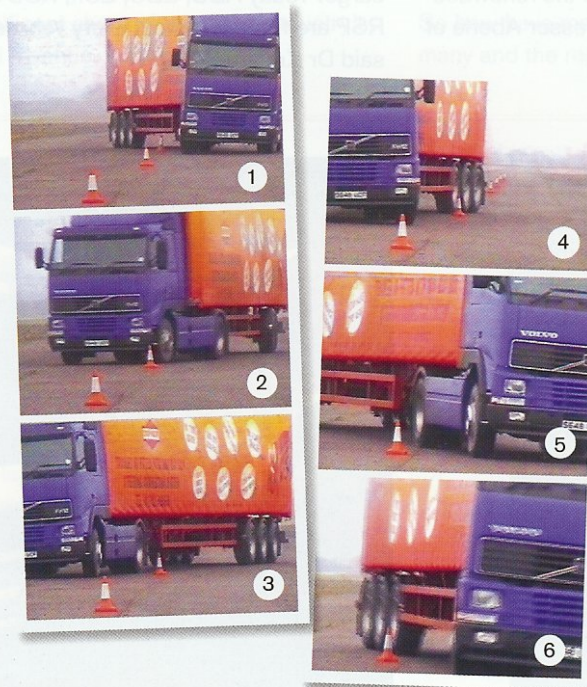
These clips show the vehicle in action. While the tractor unit steers around the first cone, the bogie remains straight. In the second slide, the tractor unit has straightened up for the next cone while the bogie is still steering around the first. This smooth manoeuvre reduces the side forces on the load and keeps the vehicle within a narrow corridor.
