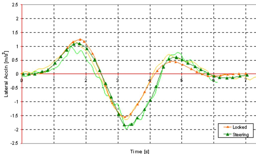
Figure 13. Trailer lateral acceleration- lane change.
