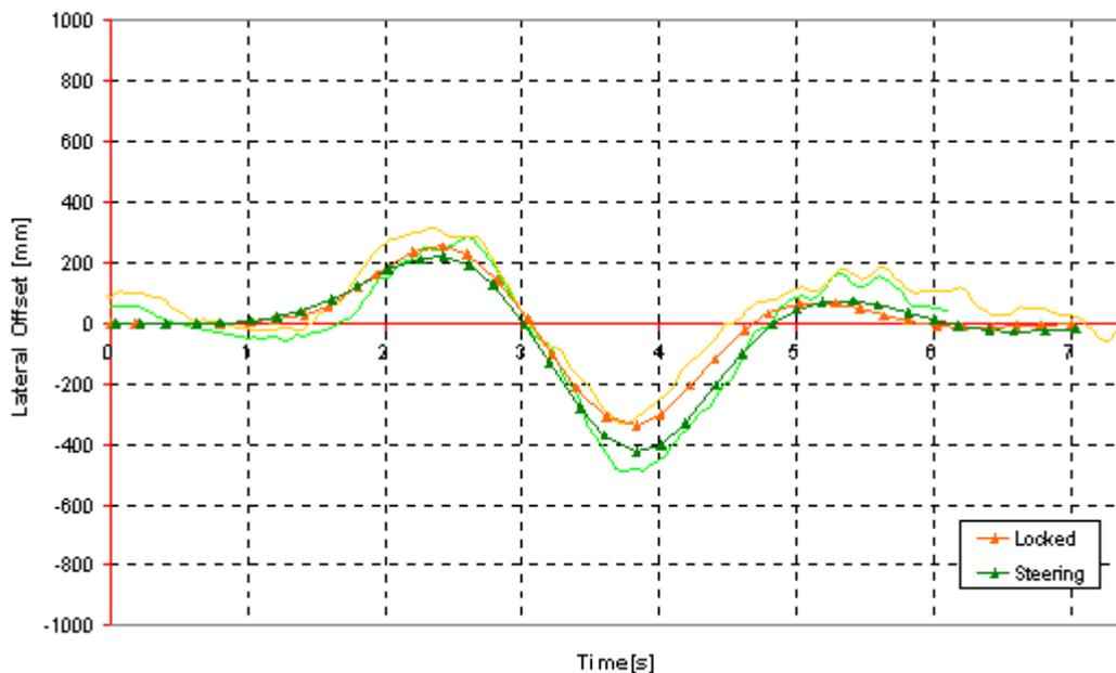
Figure 12. Lateral offset at the rear of the trailer-lane change.
