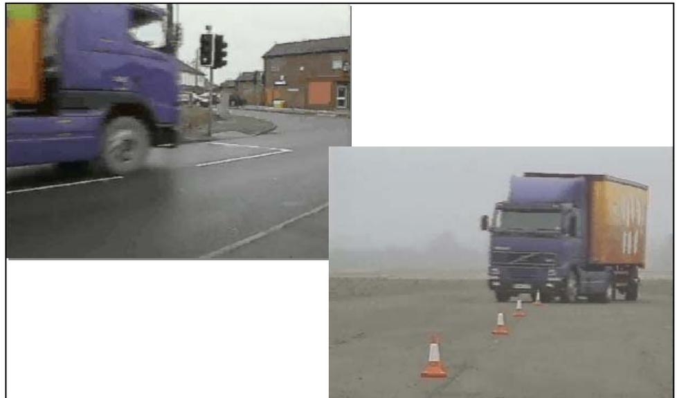
Figure 3 — SCM (16 m) semi-trailer demonstrating both low-speed manoeuvrability and high-speed stability. [http://www.silvertipdesign.com/SCM\(left\\_turn.avi](http://www.silvertipdesign.com/SCM(left_turn.avi) ./SCM(slalom).avi
